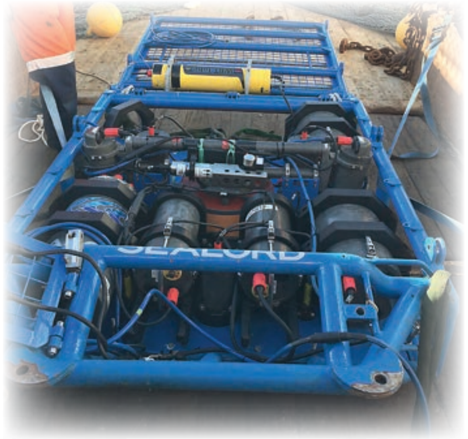
The WBT Tube installed on a subsea platform Image courtesy of CSIRO, Australia
